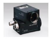
The new XC-ST Series of compact black and white camera modules offers high picture quality and excellent sensitivity. It incorporates the latest generation of CCD image sensors. The XC-ST70/CE features a 2/3-inch IT Hyper HAD CCD, the XC-ST50/CE a 1/2-inch IT HAD CCD and the XC-ST30/CE a 1/3-inch IT HAD CCD.
