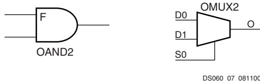
Figure 7: AND and MUX Symbols in Spartan-XL IOB
