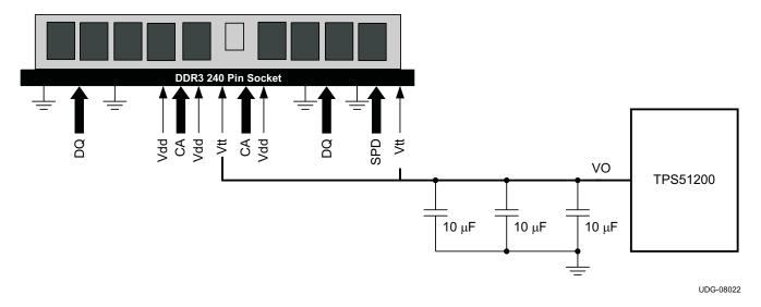
Figure 3. Typical Application Diagram for DDR3 VTT DIMM using TPS51200
