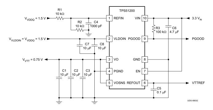
Figure 29. 3.3-V<sub>IN</sub>, DDR3 Tracking Configuration
