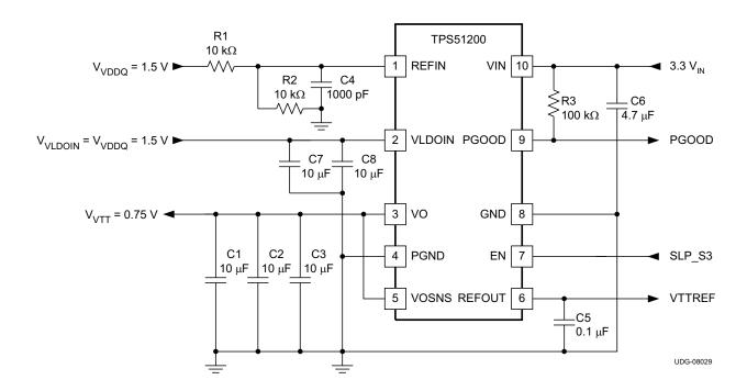
Figure 26. 3.3-V<sub>IN</sub>, DDR3 Configuration
