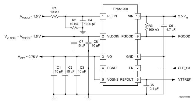
Figure 27. 2.5-V<sub>IN</sub>, DDR3 Configuration
