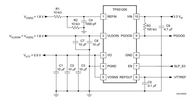
Figure 25. 3.3-V<sub>IN</sub>, DDR2 Configuration
