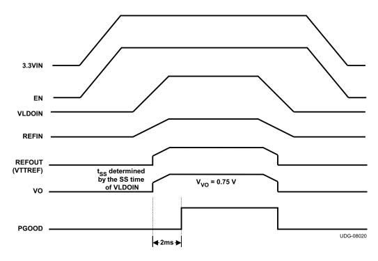
Figure 2. Typical Timing Diagram of Tracking Startup and Shutdown
