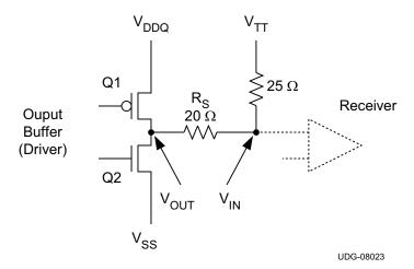
Figure 4. DDR Physical Signal System Bi-Directional SSTL Signaling
