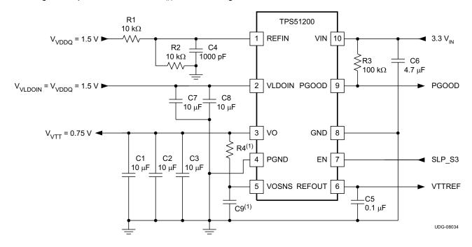
Figure 31. 3.3-V<sub>IN</sub>, DDR3 Configuration with LFP
