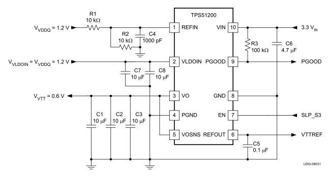
Figure 28. 3.3-V<sub>IN</sub>, LP DDR3 Configuration
