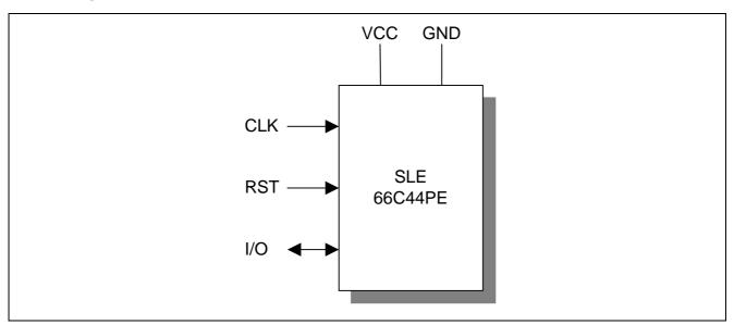
Figure 1: Pin Configuration
