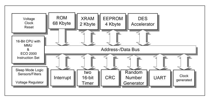
Figure 2: Block Diagram SLE 66C44PE
