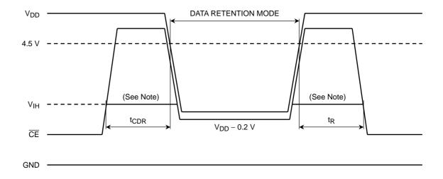
Note: When  $\overline{CE}$  is operating at the V<sub>IH</sub> level (2.4V), the standby current is given by I<sub>DDS1</sub> during the transition of V<sub>DD</sub> from 4.5 to 2.6V.
