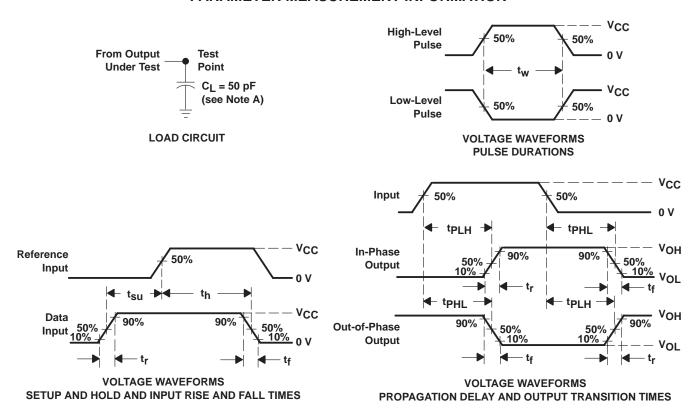
NOTES: A. C<sub>I</sub> includes probe and test-fixture capacitance.
