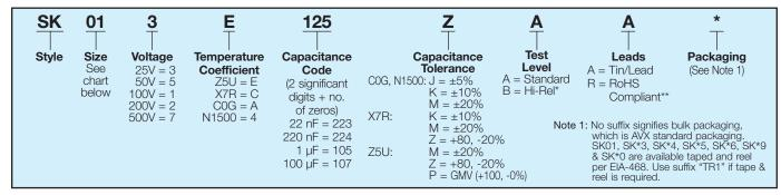
Note: Capacitors with X7R and Z5U dielectrics are not intended for applications across AC supply mains or AC line filtering with polarity reversal. Contact plant for recommendations.
