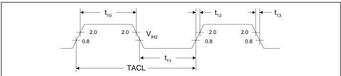
Figure 87. Pass-Thru Clock Relationship to PCI Clock
