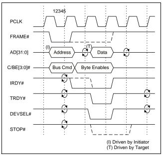
There are only two conditions where accesses to the S5920 do not return TRDY#, but assert STOP# instead. This condition is called a target-initiated termination or target disconnect. This can occur when a read attempt is made to an empty Pass-Thru FIFO. The second condition may occur when read accesses to the expansion ROM generate a retry if the nvRAM interface has not finished reading 4 bytes.
