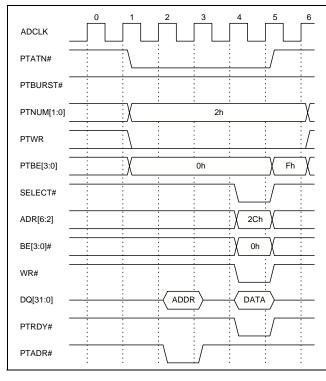
Figure 64. PCI To Add-On Passive Read
