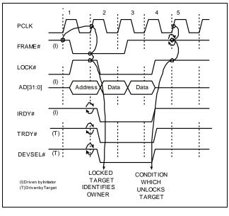
Figure 52. Access to a Locked Target by its Owner
