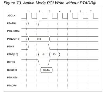
When PTADR# is active (low), the S5920 will drive the DQ[31:0] bus with the 32-bit PCI address regardless of the PTMODE pin. To avoid contention on the DQ[31:0] bus during PCI read cycles, the S5920 incorporates a turnaround cycle before starting to drive the data (DXFR# assertion). This is needed only when PTADR# is enabled and when zero wait states are programmed during a Pass-Thru read cycle. The cycle immediately following the address cycle will be a turnaround cycle as shown in Figure 13a.
