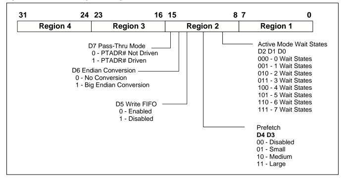
The following describes one of the four configuration registers. All four region configuration registers are exactly the same.
