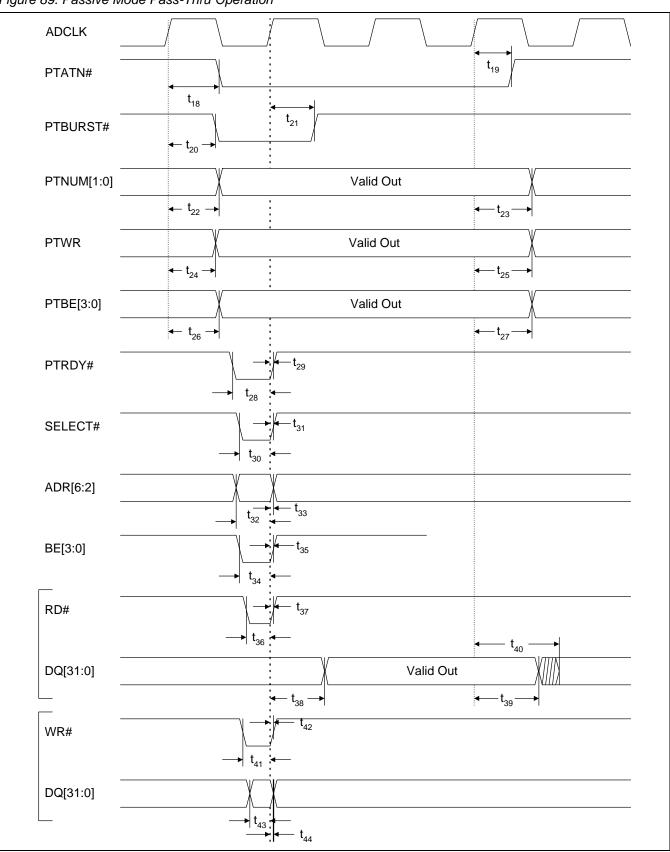
Figure 89. Passive Mode Pass-Thru Operation
