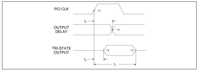
Figure 85. PCI Signal Input Timing
