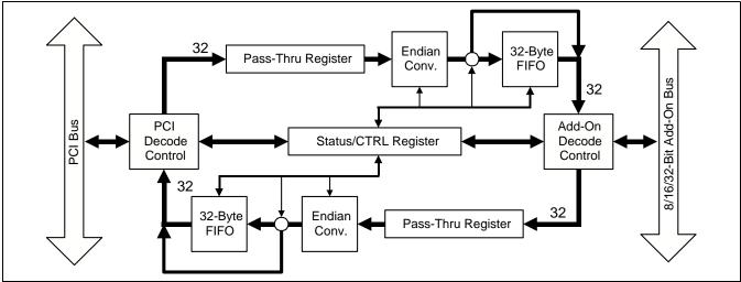
Figure 5. Pass-Thru Block Diagram
