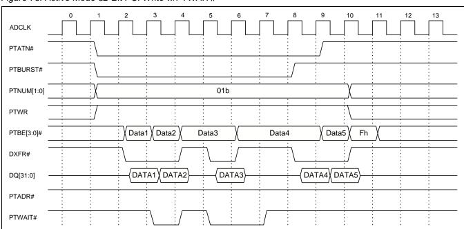
Figure 76. Active Mode 32-Bit PCI Write w/PTWAIT#
