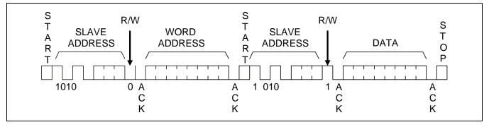
Figure 41. Serial Byte Access- Sequential Read
