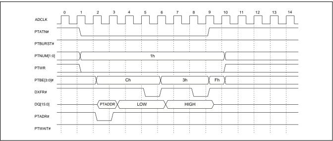
**Clock 2:** Since this region does have PTADR# enabled as an output, it is driven active (low) and the PCI address for the current transaction is presented on the DQ[31:0] bus.
