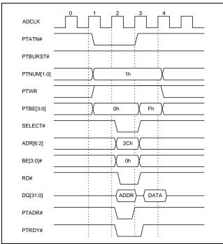
Clock 0: The address is recognized as a PCI write to Pass-Thru region 1. The PCI bus write address is stored in the Pass-Thru Address Register. The PCI bus write data is stored in the S5920 Write FIFO. Add-On bus signals PTATN#, PTBURST#, PTNUM[1:0], PTWR and PTBE[3:0] will update on the next rising edge of ADCLK.
