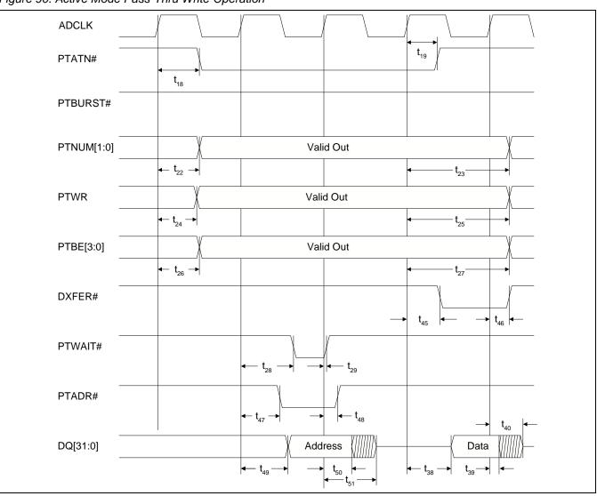
Figure 90. Active Mode Pass-Thru Write Operation
