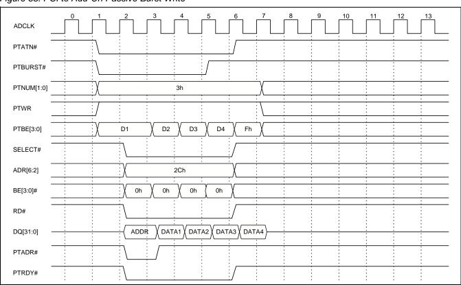
Figure 65. PCI to Add-On Passive Burst Write
