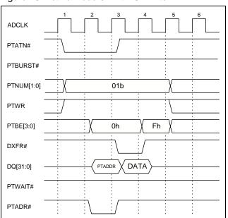
Figure 75. Active Mode 32-Bit PCI Write
