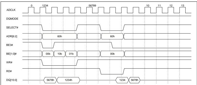
Figure 61. 16 Bit Mode Operation Register DWORD Write/Read
