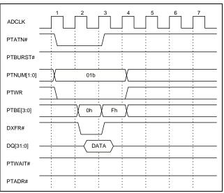
The PTADR# signal is controlled by the most significant bit of every region control field in the PTCR register. If this bit is zero then the PTADR# pin is not driven at the start of an Active mode transfer. If this bit is set to one, the PTADR# pin will be enabled and driven active (low) for one and only one clock after PTATN# was sampled active provided PTWAIT# was also sampled high.
