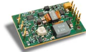
Figure 2 PKM-E 1/4-brick 25A/82.5W Size LxWxH 57.9x36.8x8.5 (12.7)mm
