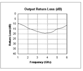
Note:- 2 SMA connectors and bondwires are included in the above data.
