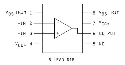
FIGURE 1. Terminal connections and logic diagrams.
