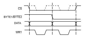
Figure 2. Write Cycles to Input Latches
