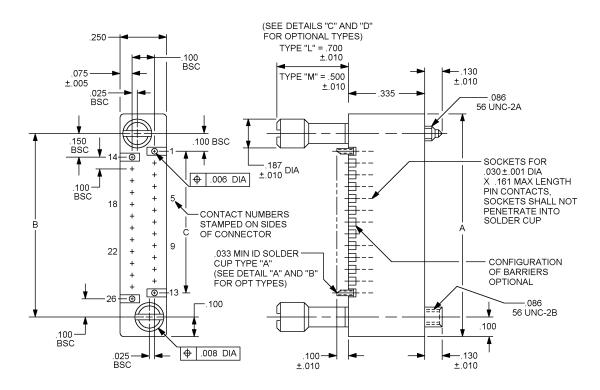
FIGURE 1. Connectors, plug, .100 (2.54 mm) spacing.
