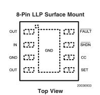
Note: The SET pin is internally disconnected for the fixed versions.
