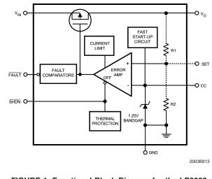
FIGURE 1. Functional Block Diagram for the LP3982
