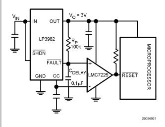
FIGURE 5. Power on Delayed Reset Application
