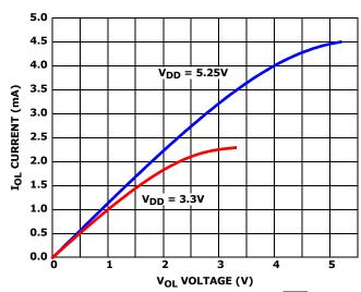
FIGURE 18.  $I_{OL}$  vs  $V_{OL}$  vs  $V_{DD}$  for  $\overline{INT}$
