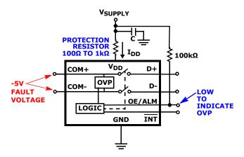
FIGURE 6. V<sub>DD</sub> SERIES RESISTOR TO LIMIT I<sub>DD</sub>
