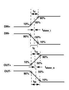
FIGURE 5A. MEASUREMENT POINTS
