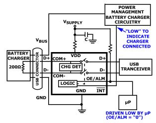
FIGURE 8. CHARGER PORT DETECTION
