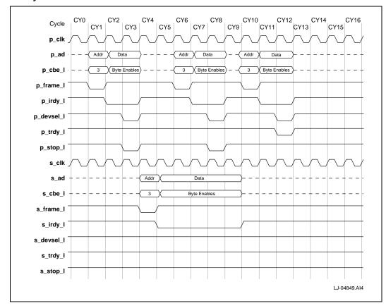
Figure 13. Delayed Write Transaction Terminated with Master Abort
