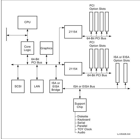
Option card designers can use the 21154 to implement multiple-device PCI option cards. Without a PCI-to-PCI bridge, PCI loading rules would limit option cards to one device. The *PCI Local Bus Specification* loading rules limit PCI option cards to a single connection per PCI signal in the option card connector. However, the 21154 overcomes this restriction by providing, on the option card, an independent PCI bus to which up to nine devices can be attached.
