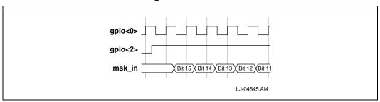
After the shift operation is complete, the 21154 tristates the gpio signals and can deassert s\_rst\_l if the secondary reset bit is clear. The 21154 then ignores msk\_in. Control of the gpio signal now reverts to the 21154 gpio control registers. The clock disable mask can be modified subsequently through a configuration write command to the secondary clock control register in device-specific configuration space.
