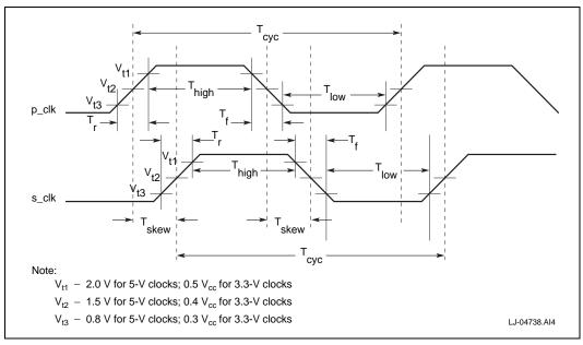
Table 43. 33 MHz PCI Clock Signal AC Parameters
