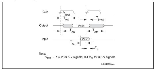
Table 45. 33 MHz PCI Signal Timing (Sheet 1 of 2)
