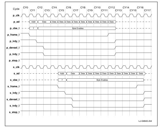
Figure 6. Flow-Through Posted Memory Write Transaction
