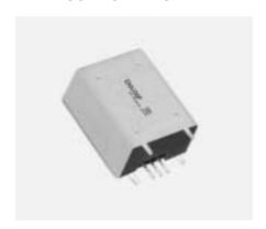
Murata Electronics' new rotational angular velocity sensor combines Murata's equilateral triangle prism vibrating unit with a revolutionary mounting technology for the piezo-electric ceramic element that produces 100 times the precision of other vibration gyroscopes.
