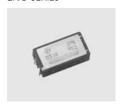
This angular velocity sensor employs the principle that a Coriolis force results if an angular velocity is applied to a vibrating object. Murata's unique ceramic bimorph vibrating unit is used as the sensor element unit, thereby enabling piezoelectric ceramics to be used for both excitation and detection. The use of this unit simplifies equipment structure and circuit configuration, thus making it possible to provide outstanding performance.
