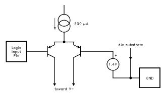
FIGURE 1. SIMPLIFIED LOGIC INPUT CIRCUITRY
