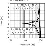
EL4421, EL4441, and EL4443 Large-Signal Response VS =  $\pm 12$ V, R<sub>L</sub> =  $500\Omega$
