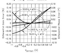
EL4421, EL4441, and EL4443 Differential Gain and Phase Error vs. Load Resistance;  $A_V=+1,\,F=3.58MHz,\,V_{OFFSET}=0\rightarrow\!0.714V$
