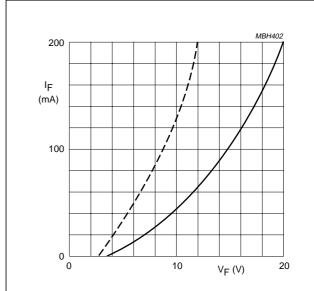
Dotted line:  $T_j = 120 \,^{\circ}\text{C}$ . Solid line:  $T_j = 25 \,^{\circ}\text{C}$ .
