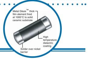
The MCHP High Reliability Surface Mount Resistors are part of the RG product family of precision resistors developed by IRC in 1960 to meet the stringent demands of the military market. In leaded form, these resistors are qualified to level S under MIL-R-39017 and MIL-R-55182. The MCHP resistor utilizes the core element from this series, but with modified contacts and encapsulation.
