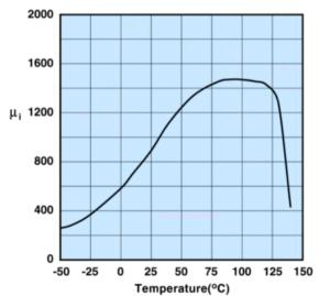
Measured on a 17/10/6mm toroid at 100kHz.
