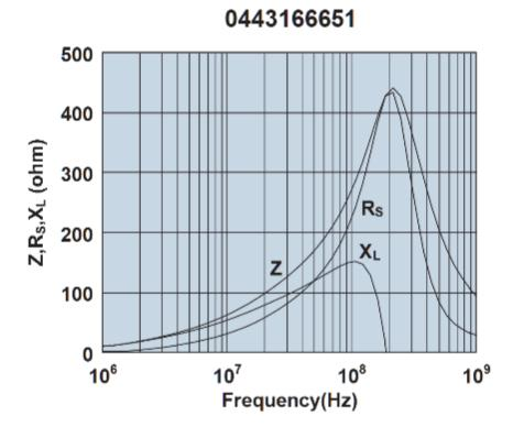
Impedance, reactance, and resistance vs. frequency.
